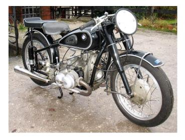
The engine in this special is one of his engines. It is 773 cc, compression ratio 8.4:1 and has 44 mm inlet valves. The internals have been extensively reworked, including polishing and much piston reworking. The early military machines had a rather hot camshaft, which was soon replaced by a softer version.
