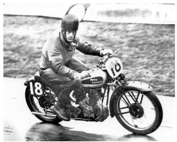
Booker is pictured here at the 1934 Donington August Bank Holiday meeting. This machine has a standard petrol not the "proper" works tank. Going down to the Melbourne Hairpin at Donington, Booker's bike was capable of 103 mph, and could keep up with the works 350 Norton's, not bad for a 1934 push rod 250. Booker himself gave me much of this information.
