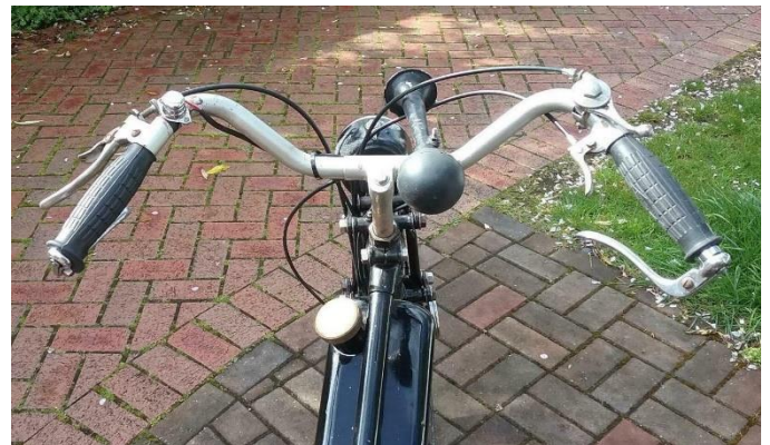
The controls of a 1950 New Hudson Autocycle.
