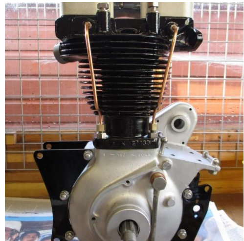
Rocker Box Drains.
