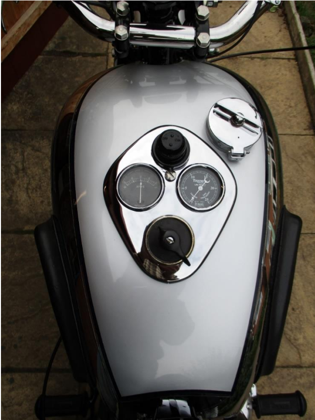
Restored instrument panel with the correct oil pressure gauge needle.
