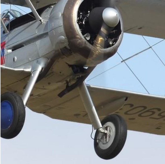
A close-up image of the Gloucester Gladiator undercarriage. It can be seen that the wheel moves vertically on the stub axle.
