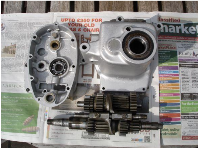
Gear Box prior to assembly.
