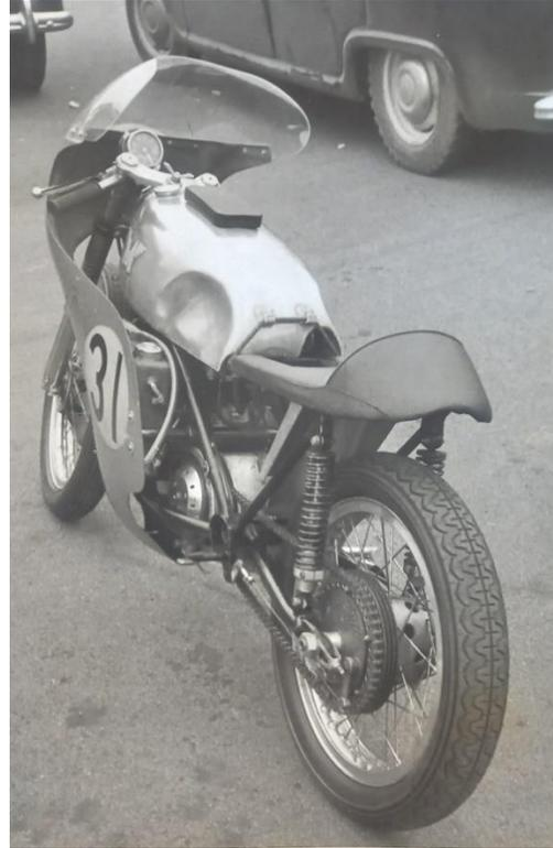
A Matchless with pannier tanks in the fairing and fuel pumped up to the header tank by the swing arm. Norton type frame, built by Bob and Joe Potts. It's still running at events like Goodwood but radically altered.
