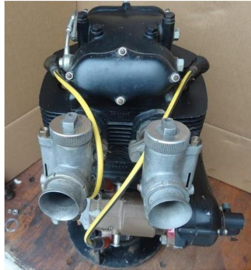
The pictures show some neat external modifications but no details of the internals were given. The advert states that the engine was built at the BSA experimental centre and after the TT Chris messed around with the bore and stroked and raised the capacity to near 750cc. He then put it in his grass combo. Later it was paraded at some shows, notably Stafford.
