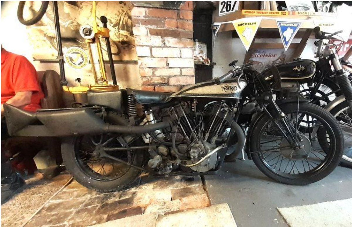
1928 Norton fitted with a 1927 JAP 1000cc racing engine. Built for Brooklands. It's been in Jack's family since 1936.
